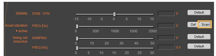
When operating, the frequency analysis can be started anytime. But because the current of the motor is being analyzed for the frequency analysis the, the output stage must be turned on. As soon as the analysis is completed, the measuring results are shown in WebMotion® and the frequency can be set.
