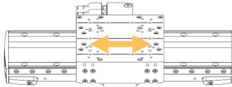
With the START the LINAX® or ELAX® linear motor will be referenced automatically and will then move the distance back and forth that was indicated manually by hand before.
