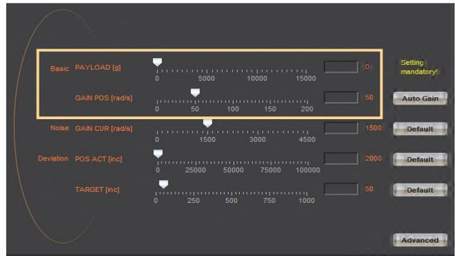
Bandwidth of position controller      GAIN POS
