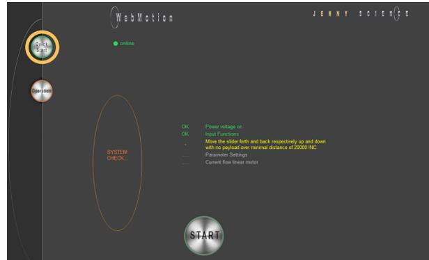
In order to test the functionality of the measuring systems the system asks you to move the slider of the LINAX® linear motor axis of a distance of at least 20mm back and forth.
