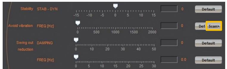
When operating, the frequency analysis can be started anytime. But because the current of the motor is being analyzed for the frequency analysis the, the output stage must be turned on. As soon as the analysis is completed, the measuring results are shown in WebMotion® and the frequency can be set.
