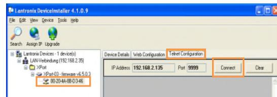
Click on IP-address, choose „Telnet Configuration“, press “Connect” button and confirm with “Enter” key.
