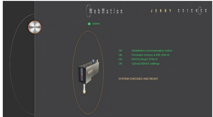
If the XENAX® servo controller does not recognize a LINAX® or ELAX® linear motor axis or a ROTAX® rotary axis, XENAX® assumes a connection with third party motor. Instead of “Go Pos 0” WebMotion® offers Jog + und Jog – functions.
