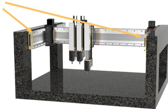
When switching on the system, these two Y-axes have to be aligned in order to move without mechanical tension.
