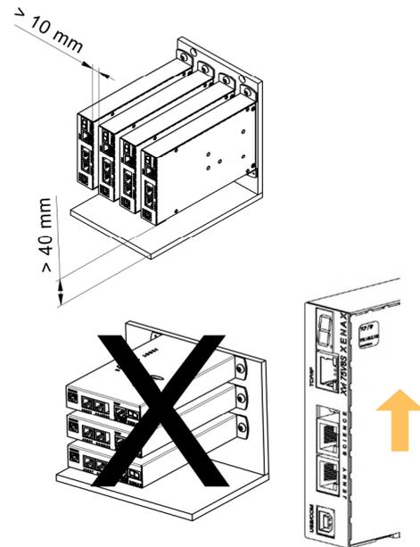
When operating with a power supply motor above 60VDC, the XENAX® Servo controller must be mounted in an electrical control cabinet and the XENAX® Servo controller must be connected to protective earth using the shielding clamp (Art. No. 130.09.00) for motor cable.
