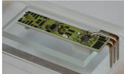
With the ELAX® linear motor slide and the XENAX® servo controller the ball shall be touched and the touching position detected. The touching position is the offset of the actual force curve measurement. This offset compensates the height tolerances of the different measuring objects.
