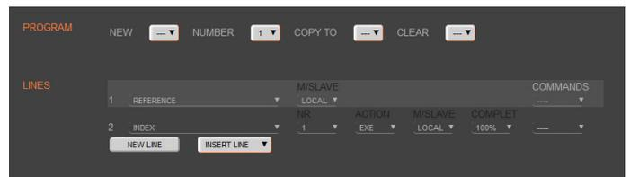
If reference position differs from starting position, an index (INDEX 1) can be executed to move to start position.
