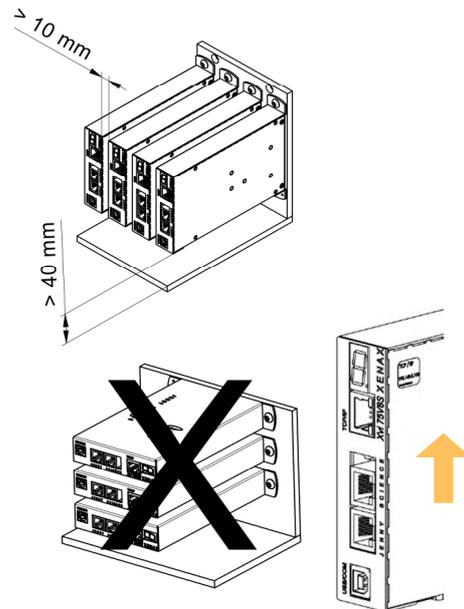
It is recommended to install the XENAX® servo controller in a control cabinet and to connect the motor cable to the protective earth using the EMC shield clamp (Art. No. 130.09.00).
