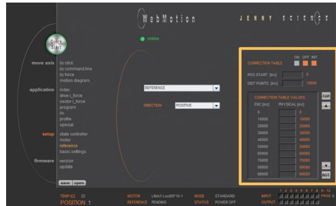
The range for the way can be freely selected. Furthermore, the starting point and the distances between the entries of the table can be defined. If for example the range 0-100'000 increments shall be corrected, the starting position is 0inc and the distance for the 50 remaining table entries is 2'000 inc (100'000 / 50).
