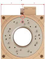
For the alignment of the rotor flange, a single bore Ø4H6 with aligned marking on the shaft and a marking on the symmetry axis of the housing is provided. The absolute zero point is in straight alignment of the two markings.
