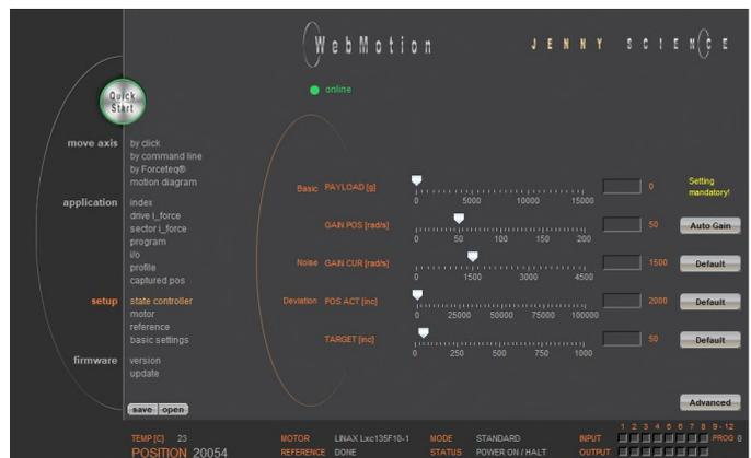
The screenshot shows the 'Basic' settings page in the WebMotion software. The 'Basic PAYLOAD [g]' parameter is set to 0. The 'GAIN POS [rad/s]' parameter is set to 50, with an 'Auto Gain' button next to it. Other parameters include 'Noise GAIN CUR [rad/s]' at 1500, 'Deviation POS ACT [rad]' at 2000, and 'TARGET [rad]' at 50. The interface also shows a 'Quick Start' button and a 'Save/Open' button.
