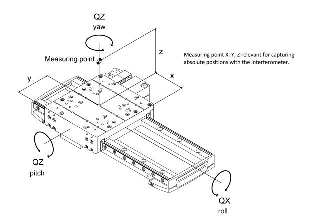
The LINAX<sup>®</sup> Lxs linear motor axes are delivered with the following tolerances as standard. The specifications are based on an unloaded condition.
