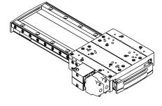
Lxs mechanical zero point according to REFERENCE: Carriage positioned 1.5mm from the stop on the right, when viewed from the connector housing.
