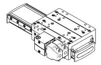
Lxu absolute zero point according to REFERENCE: Slider extended towards the connection cable
