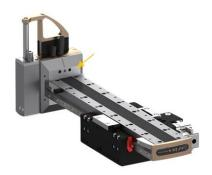
There can be mounted a further Lxu or a Lxc linear motor axis on the front of the LINAX® Lxu. If the front plate is removed, the front flange Lxu can be mounted with 4 screws and 2 centering pins. These front flanges can be rotated, mounted and centred in a 90 pattern (except from ELAX®).
