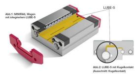
The most recent used guiding carriages are maintenance free and no re-lubrication is necessary. The reservoir at the inside of the carriages lubricates all the balls automatically. Even for short-stroke applications lubrication is ensured.
