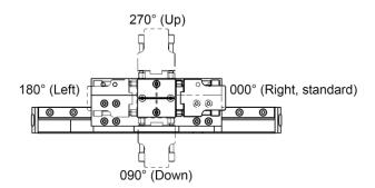
Lxs and Lxu Rotary connector case in 90° pattern Default cable connector directed to the right
