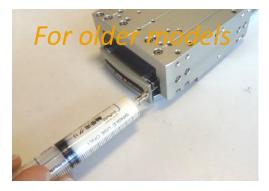
For the Lxu, Lxs and Lxe types we use ball bearing guides with integrated permanent lubrication. For the older LINAX® models re-lubrication was completed with a lubricant filled syringe in order to refill the internal lubrication reservoir. Depending on dynamics the re-lubrication was suggested every 12 months.
