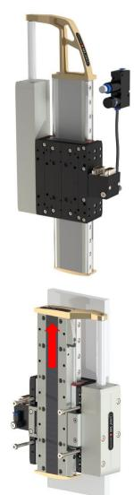
This weight compensation for the Lxu axis is also based on air pressure, while there is no air consumption. The air connection of weight compensation is located on the connector case to save room and to keep cables one-sided. With a customary air pressure regulator e.g. Festo "VRPA" the compensation force can be adjusted until the slider holds position or moves upwards in case of power interruption.
