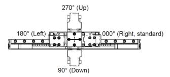
Lxs and Lxu Rotatable connector housing in 90° increments Standard cable outlet to the right when viewed from the connector housing.
