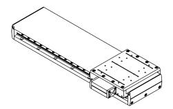
Lxe absolute zero point according to REFERENCE: Slider extended towards the connection cable
