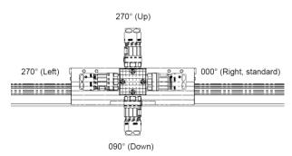
Lxs and Lxu Rotatable connector housing in 90° increments Standard cable outlet to the right when viewed from the connector housing.
