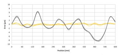
Measurement system 1 $\mu$ m optical, relevant measurement point 150mm above the scale
