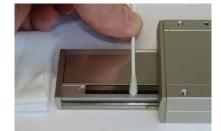
After mechanical mounting or if there is visible dirt, the class scale should be cleaned thoroughly. Please do not touch glass scale afterwards.
