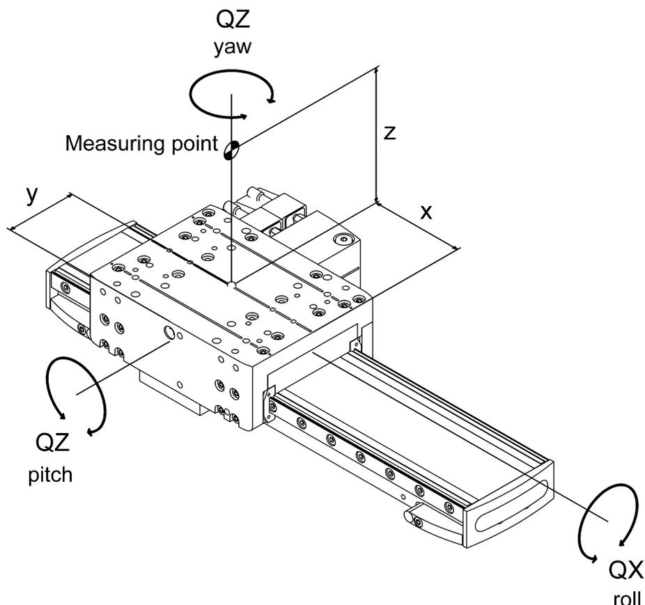
The LINAX® Lxu linear motor axes have following tolerances as a standard. These data is based on measures with linear motors free of load.
