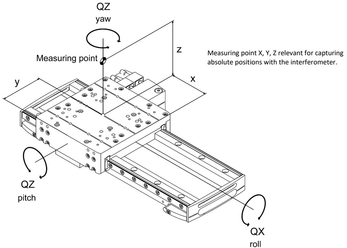
The LINAX® Lxs linear motor axes are delivered with the following tolerances as standard. The specifications are based on an unloaded condition.
