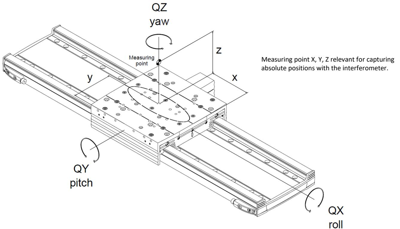
The LINAX® Lxs linear motor axes are delivered with the following tolerances as standard. The specifications are based on an unloaded condition.
