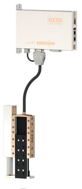
Forceteq® Basic offers a current-based force measurement technology that is seamlessly integrated into the XENAX® Xvi servo controller. No external sensors are required, enabling real-time monitoring and recording of force-displacement diagrams, leading to improved production quality and higher throughput.
